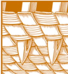
Branded backings provide a foundation that eliminates needle deflecting yarn damage, providing crisp pattern definition and greater appearance retention.
