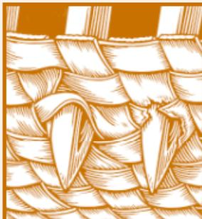
Commodity level backings have a high incidence of needle deflection causing yarn damage and poor pattern definition.
